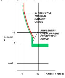
High AC voltage shutdown (59) - Output voltage on any phase exceeds preset values. Time to trip is inversely proportional to amount above threshold. Values adjustable from 105-125% of nominal voltage, with time delay adjustable from 0.1-10 seconds. Default value is 110% for 10 seconds.
